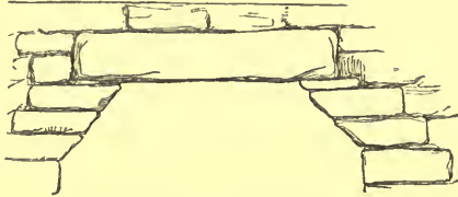
Fig. 5. Horizontal arch of the door, as seen from within the cell.
